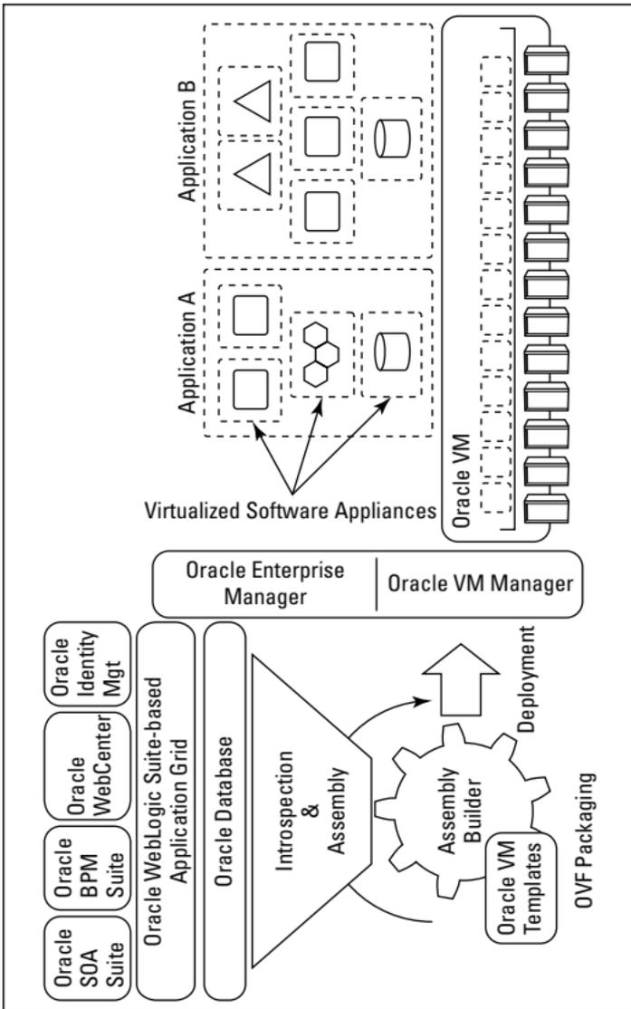
**Figure 3-3:** Oracle Virtual Assembly Builder.
