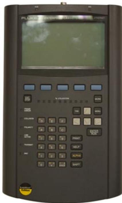
**A LAN Analyzer has all the functions of the previous tools we looked at, but its output is geared to the network professional—you.**
