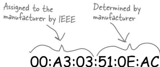
A MAC address is assigned to every device connected to an Ethernet network. In your computer, that is the network card. The beginning part of the MAC address designates the manufacturer. The later part, the manufacturer increments, so all their products have unique MAC addresses. It is like a social security number, in that you really can't tell where a person lives just by looking at it.
