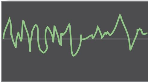
A logic analyzer may detect a few 1's and 0's but this is real noisy signal
