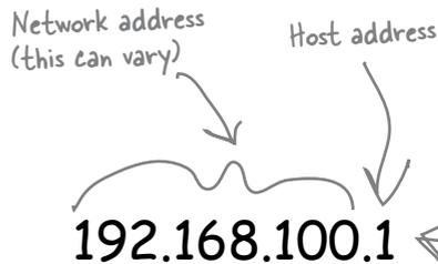
A IP address is made up of a network address and a host address. The host part is the unique bit assigned to a particular network device. It is much like a phone number, which has a country code, area code, and local calling area—finally, your unique individual number.
