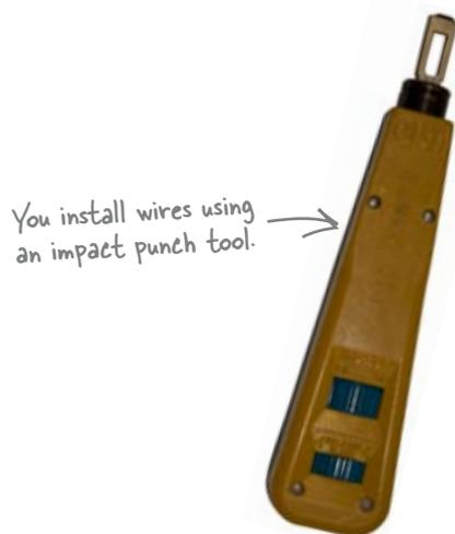
The way in which you install the wires is important. The wires follow a specific color pattern, and you need to follow this so that you can make connections between devices. The pattern depends on the type of block you're using and the type of wire you're punching into the block.
