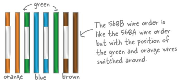
Can you see any similarities between the 568A and 568B wire orders? The order for each standard is basically the same except the orange and green wires are switched over.
