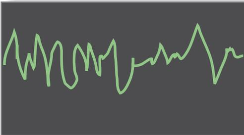
This is just noise. A cable too close to a power line or some other type of signal source could cause this. Even a bad or incorrect connection could cause this signal.
