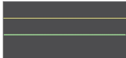
The oscilloscope shows a clear and distinct signal, but as it always falls below the logical high voltage level, the logical analyzer interprets it as a constant 0.
