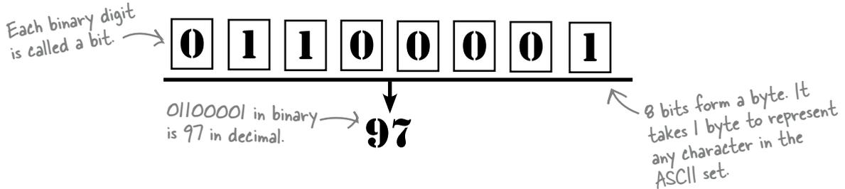
Each byte needs to be translated to an ASCII character. To do this, we convert each byte into its decimal equivalent, and then look up the corresponding ASCII in an ASCII table, just like the one in Appendix ii.
