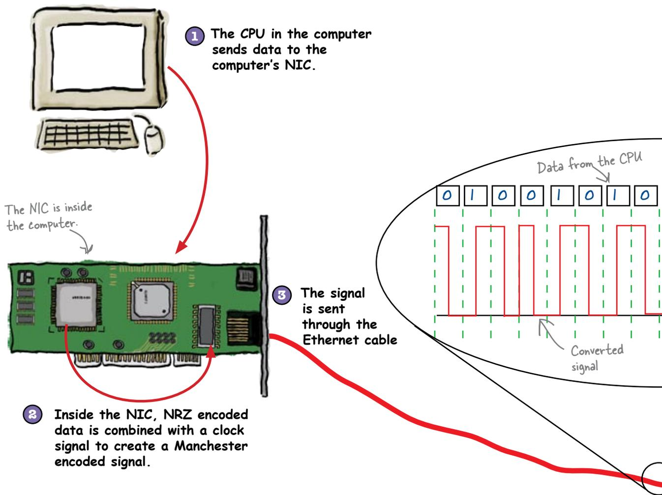
The protocol for 10BaseT Ethernet specifies that the signal will be encoded using Manchester encoding.
