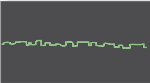
This is a real signal, but the voltage level is very reduced. A really long cable could cause this as well as bad connectors.
