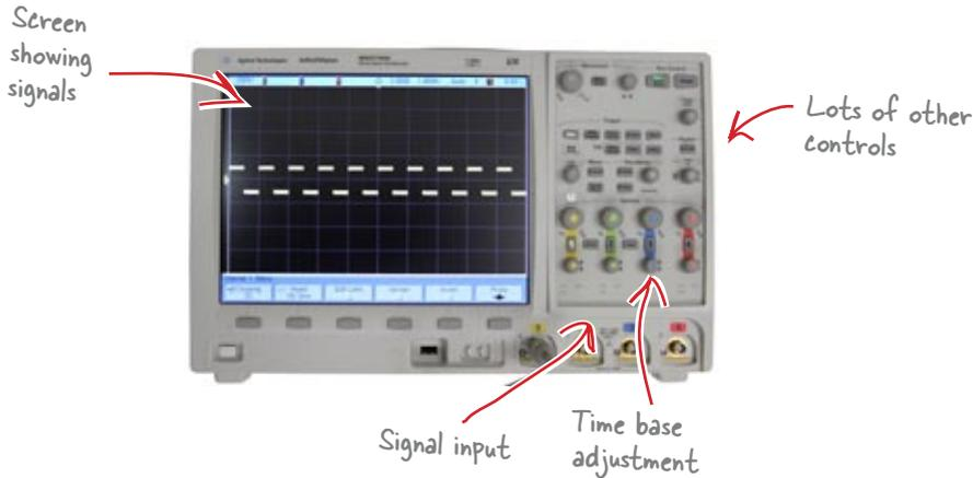
**This is the same oscilloscope we saw earlier, but it can work as a logic analyzer as well. Yes, it's very expensive.**
