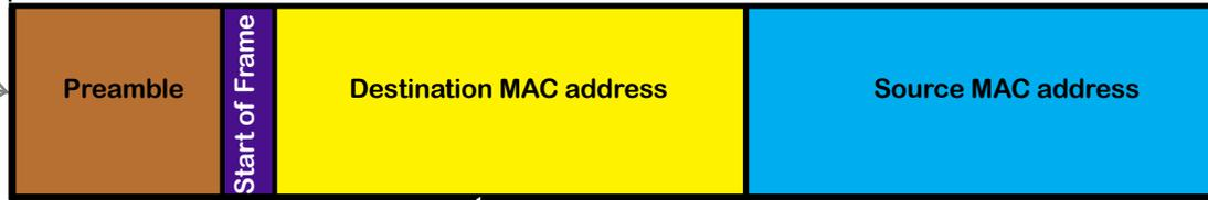
The SOF is one byte long and ends with two ones: 10101011. The SOF tells the receiving device that the crucial content of the frame is on its way.
