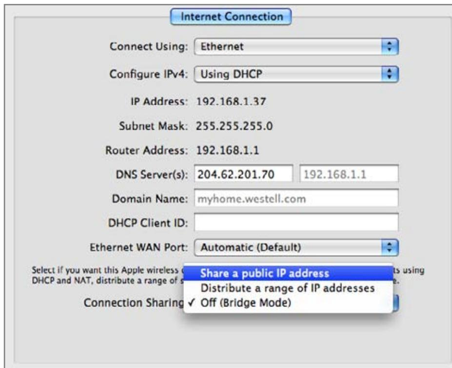
Configuring **NAT** on most access points consists of turning it on, and that's about it.
