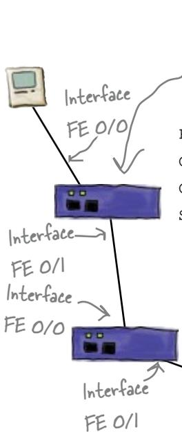
For the client connected to this router to send traffic to the other client, this router needs to know how to send traffic to the 192.168.102.0 network.
