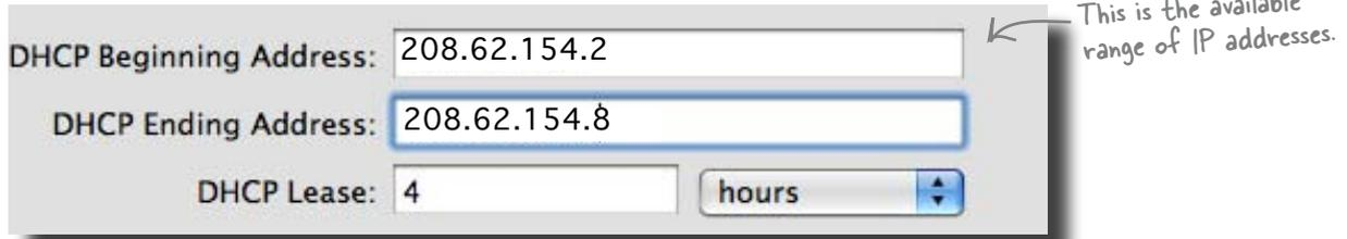
But what happens when we have more clients than available IP addresses? The DHCP server can only give out a limited range of IP addresses, and when it runs out, that's it. It can't offer any new clients a connection. So what can we do to get around this?
