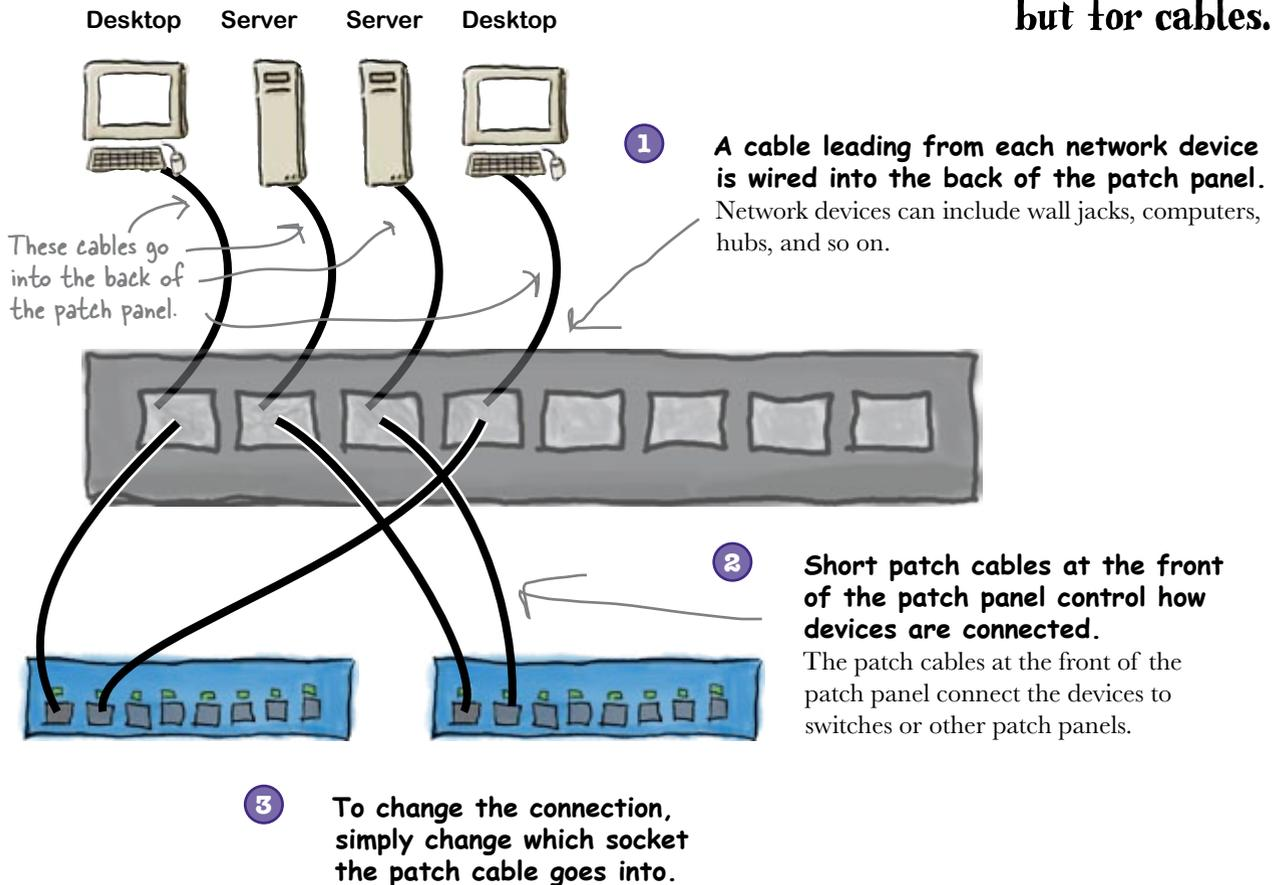
If you use a patch panel, it means that it's much easier to change the connection between two devices. All you need to do is change which socket the patch cables at the front are connected to, so the patch panel gives you an easier interface for managing connections.
