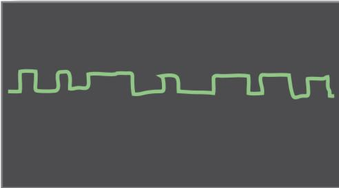
This is a real signal. It represents data in the form of 1's and 0's which correspond to the high and low voltages.
