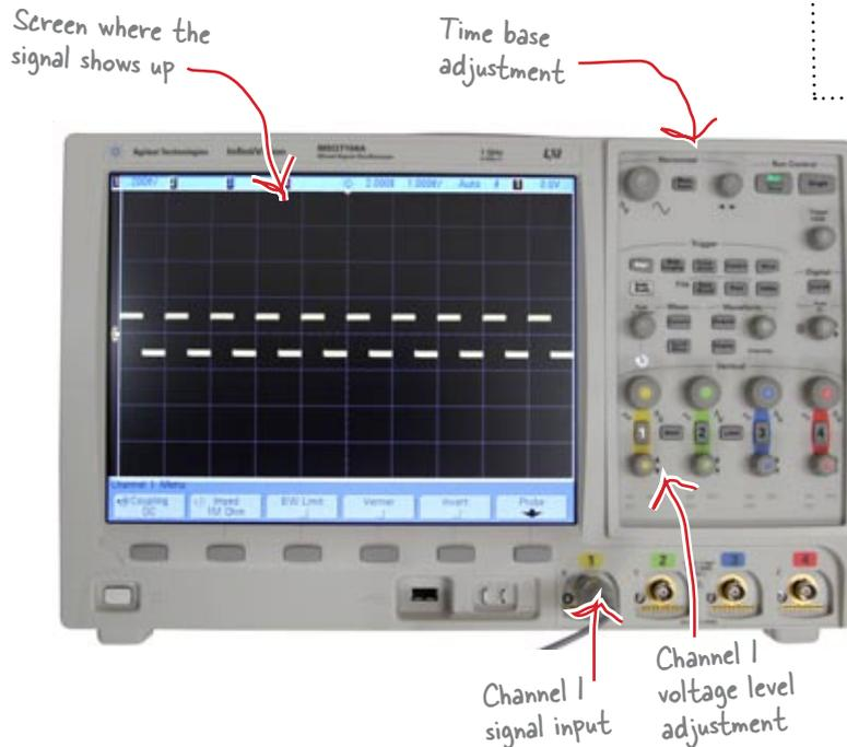
Here's an example readout from the oscilloscope showing you the voltage changes in a cable over time.
