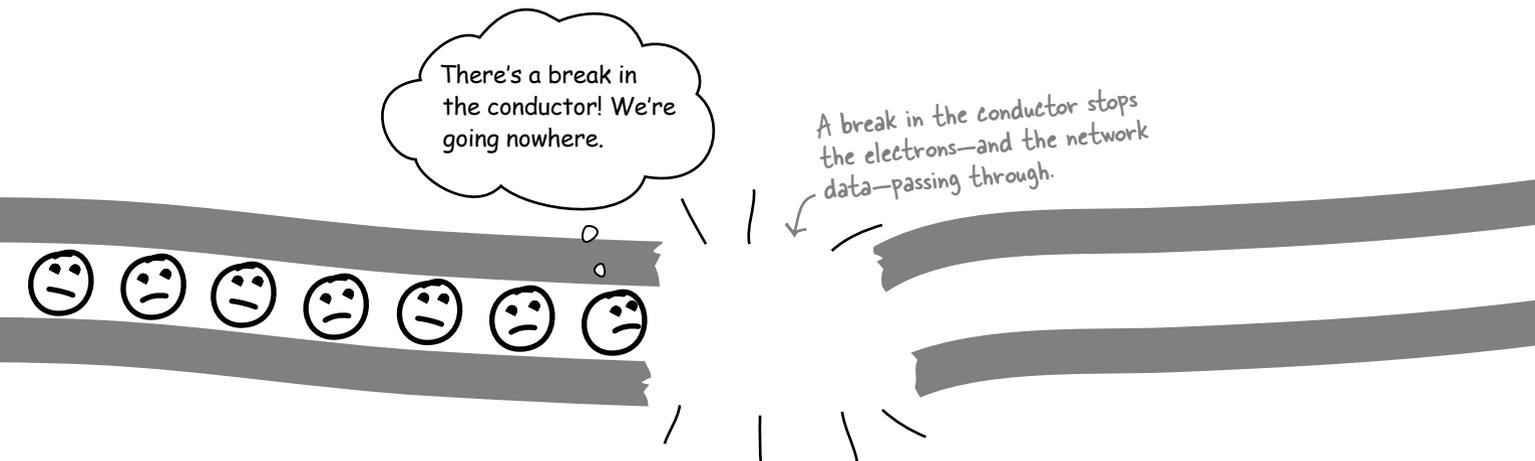
This means that if there's a break in the coaxial conductor of the bus, Coconut Airways will get network error messages.
