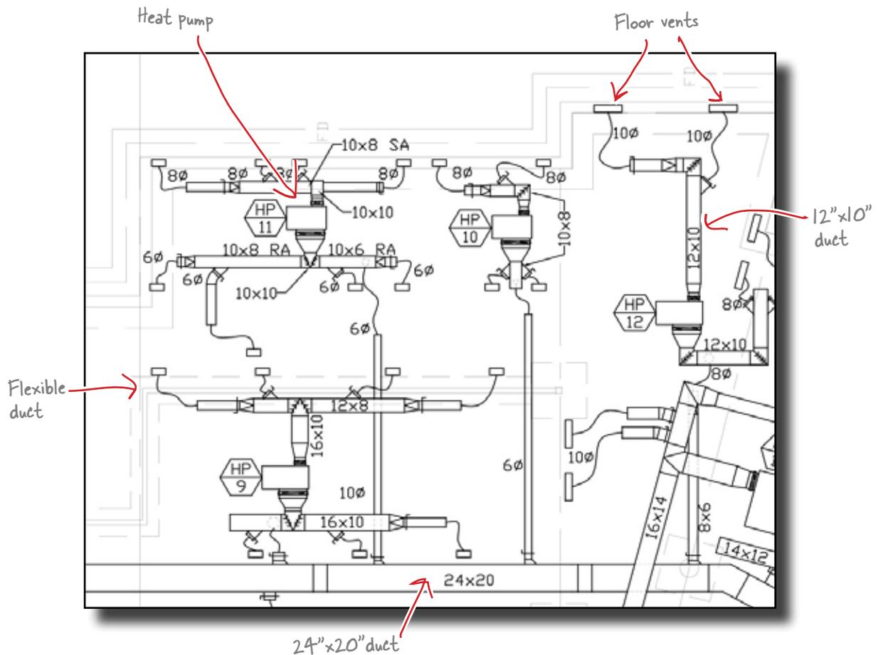
Most of this ductwork will hang via hangers from the floor joists, hanging down about 2'.
