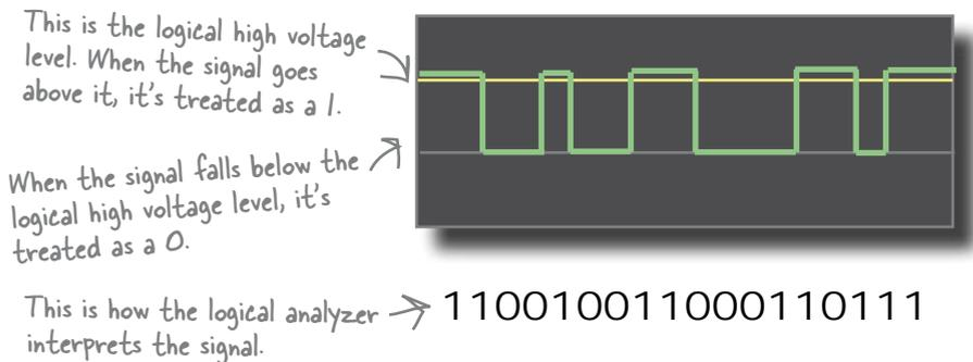
The voltage changes in the signal represent data in the form of binary numbers, so a logical analyzer allows you to see the stream of data based on the logical voltage level. It effectively allows you to see the data in the signal.
