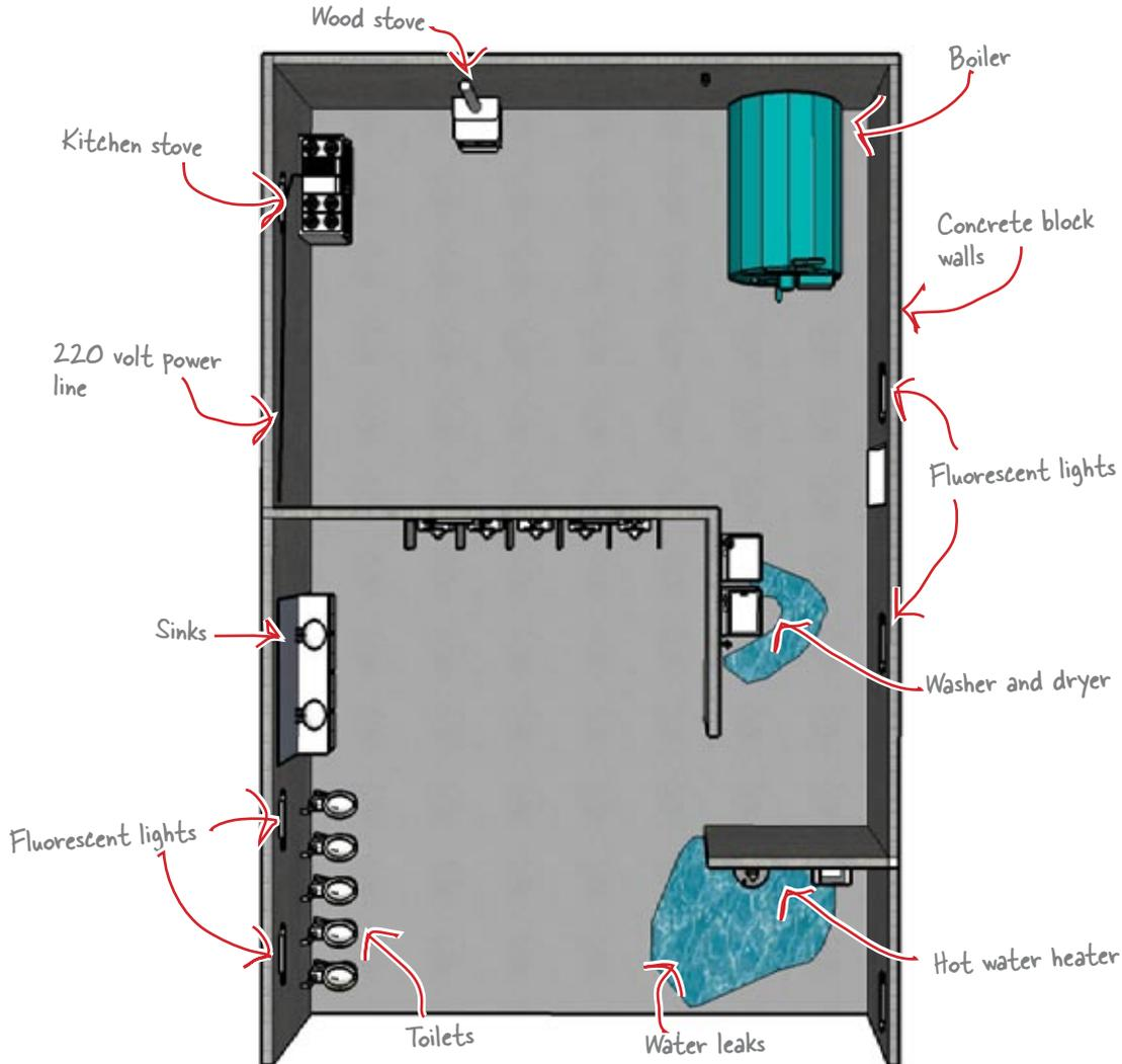
Notes: The boiler may create heat and vibrations, so might the laundry equipment. There also may be water around the laundry equipment. The large electrical line needs to be avoided. The hot water heater and wood stove will be hot and need to be avoided. The fluorescent light may cause some interference.
