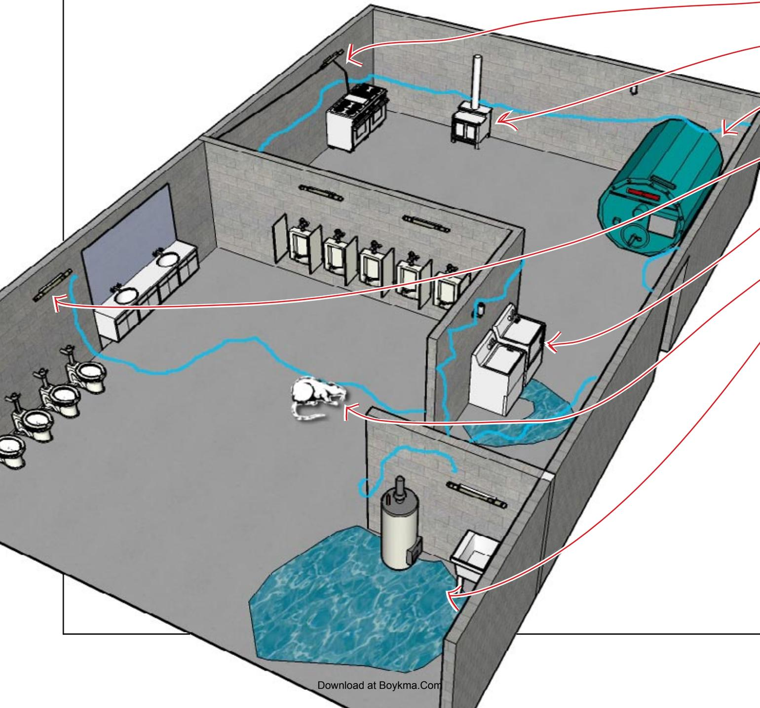
Be careful where you run cable. Power lines interfere with network cable signals.
