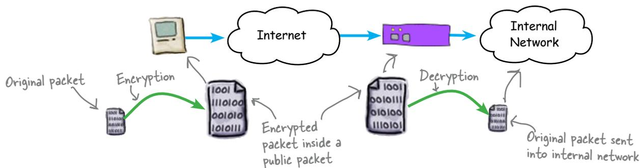
VPN works by encrypting the packets destined for the internal network. It then puts those encrypted packets into the data section of a regular TCP packet, sends that packet across the public network, and then the VPN gateway removes the encrypted packet, decodes it and sends it into the internal network.
