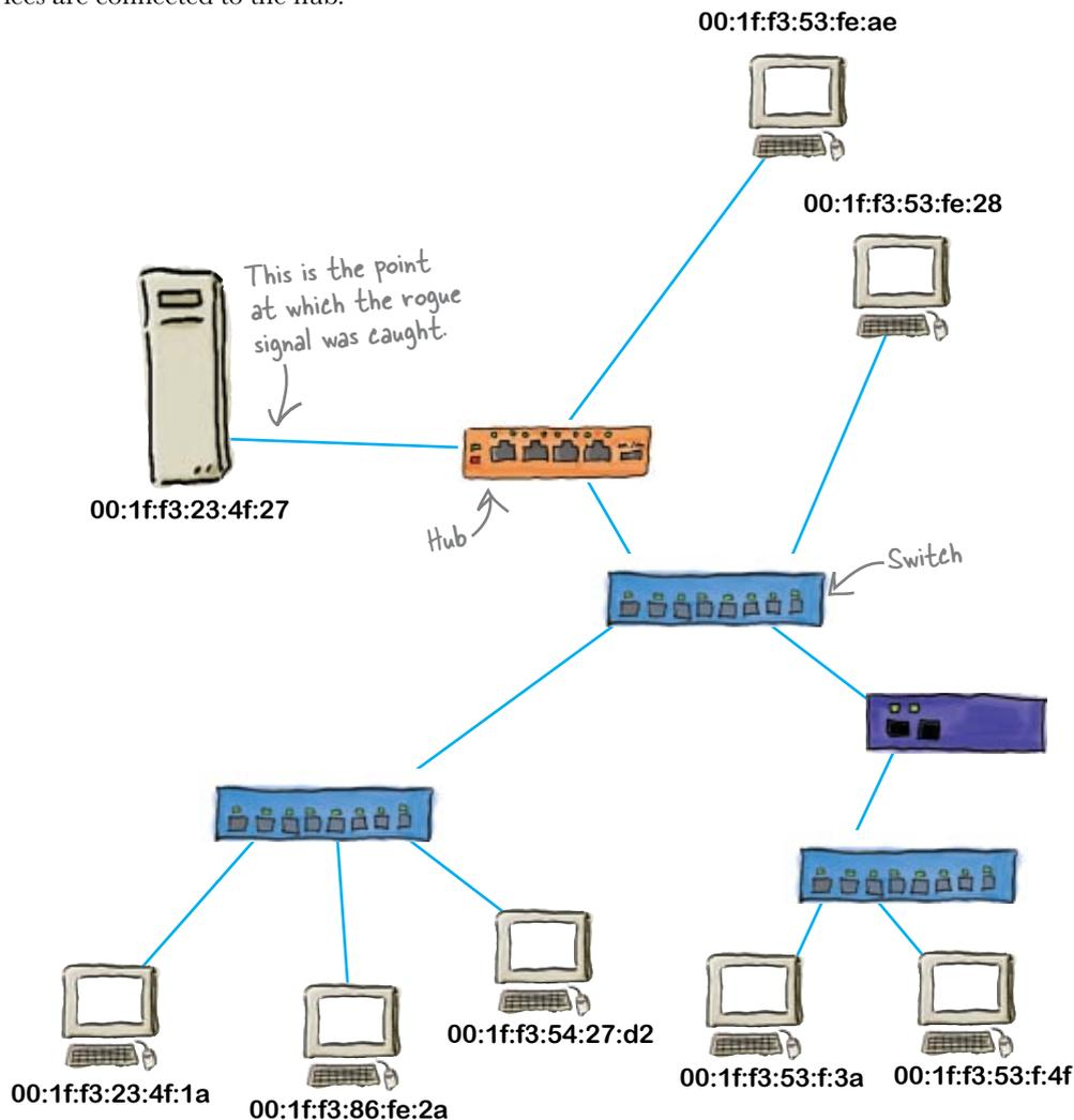
The hub has two devices connected to it that could have sent the signal, a computer and a switch. As the computer MAC address doesn't match the one we're looking for, we know the computer didn't send the signal; it must have been the switch.
