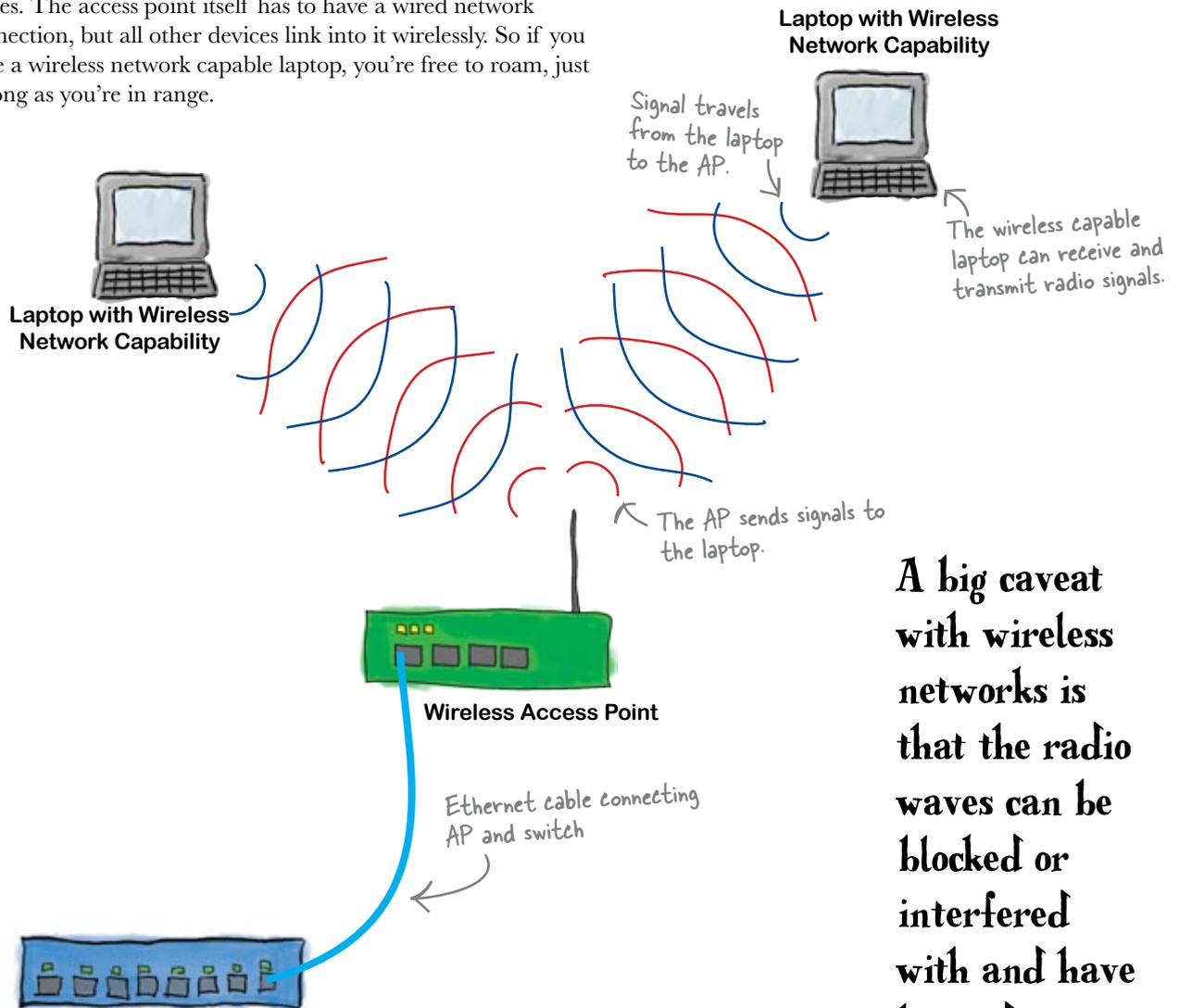
**A big caveat with wireless networks is that the radio waves can be blocked or interfered with and have limited range.**
