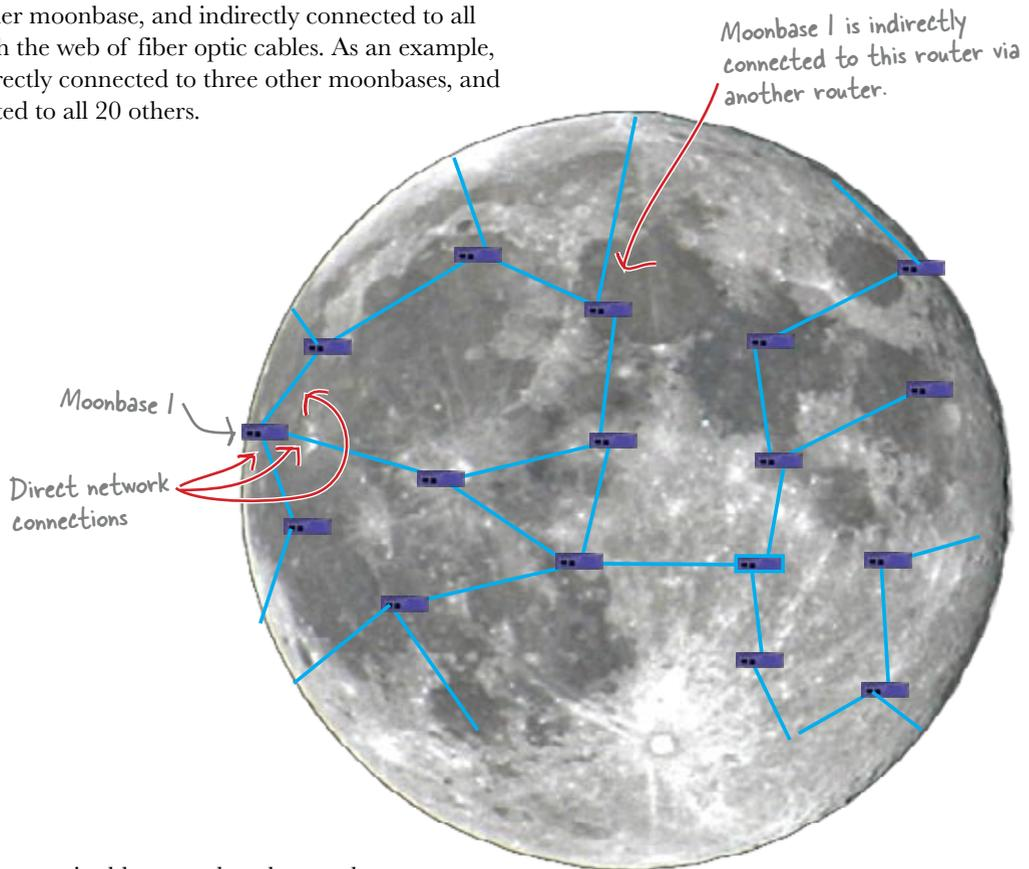
The Moonbase 1 router is able to send packets to the moonbases it's directly connected to, but it can't communicate with any of the other 18 moonbases it's only connected to indirectly.
