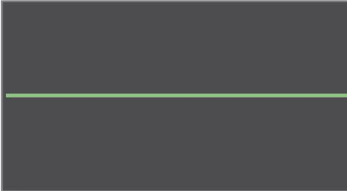
There is no signal here. So the cable could be broken or just not connected.
