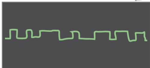
...and a network signal distorted by noise on the wire.
